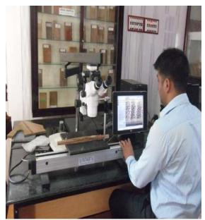
Figure 4: Measurement of tree ring width and vessel area in core sample of teak.
