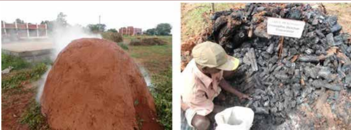
Heap method of biochar preparation in Tamil Nadu (Source: Jeyaraman, TNAU)
