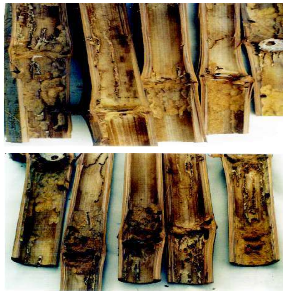
Internal damage of bamboo culms done by Phloeobius crassicollis
