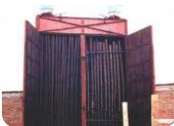
Culms stacked in a heating chamber
