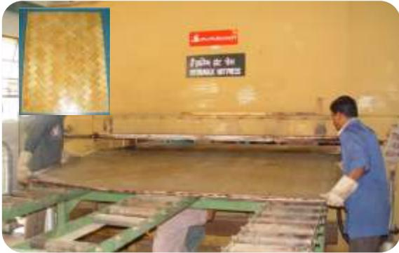
Fig. 11.2 : Hydraulic hot press for manufacture of BMB
