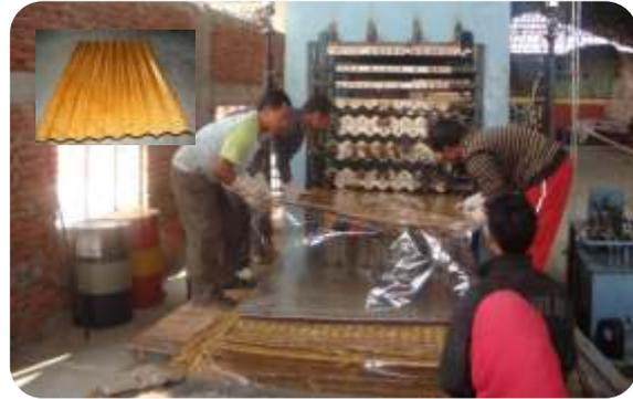
Fig 11.3: Hydraulic hot press for manufacture of BMCS
