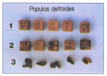
Termite resistance obtained by Zinc borate treatment, (1) and (2) treated, (3) is control
