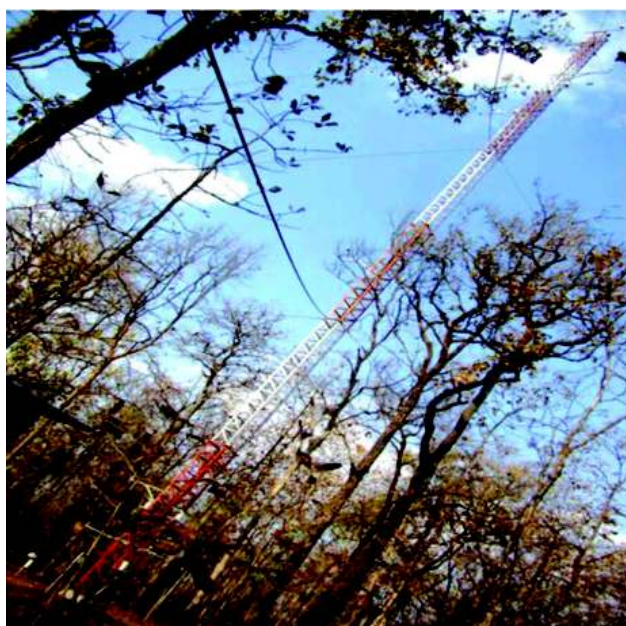
Carbon Flux Tower
