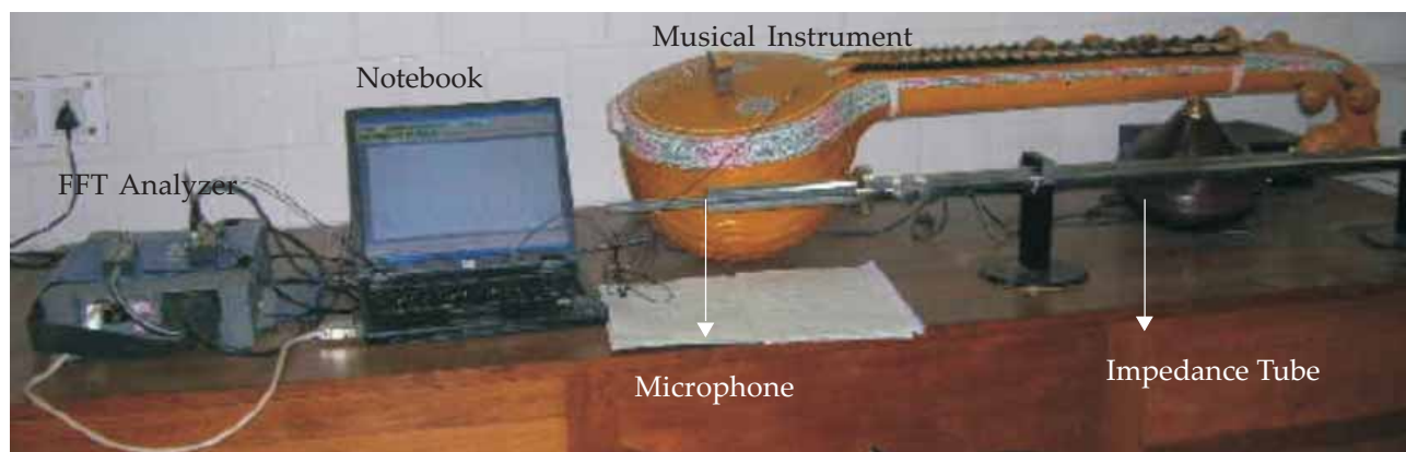
Acoustic measurement unit to detect the sound waves of musical instruments
