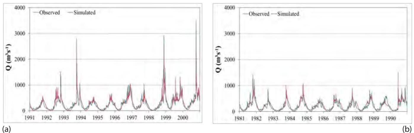
**Figure 10.4:** Observed and simulated hydrographs at the Ban Don station for the (a) calibration and (b) validation periods
