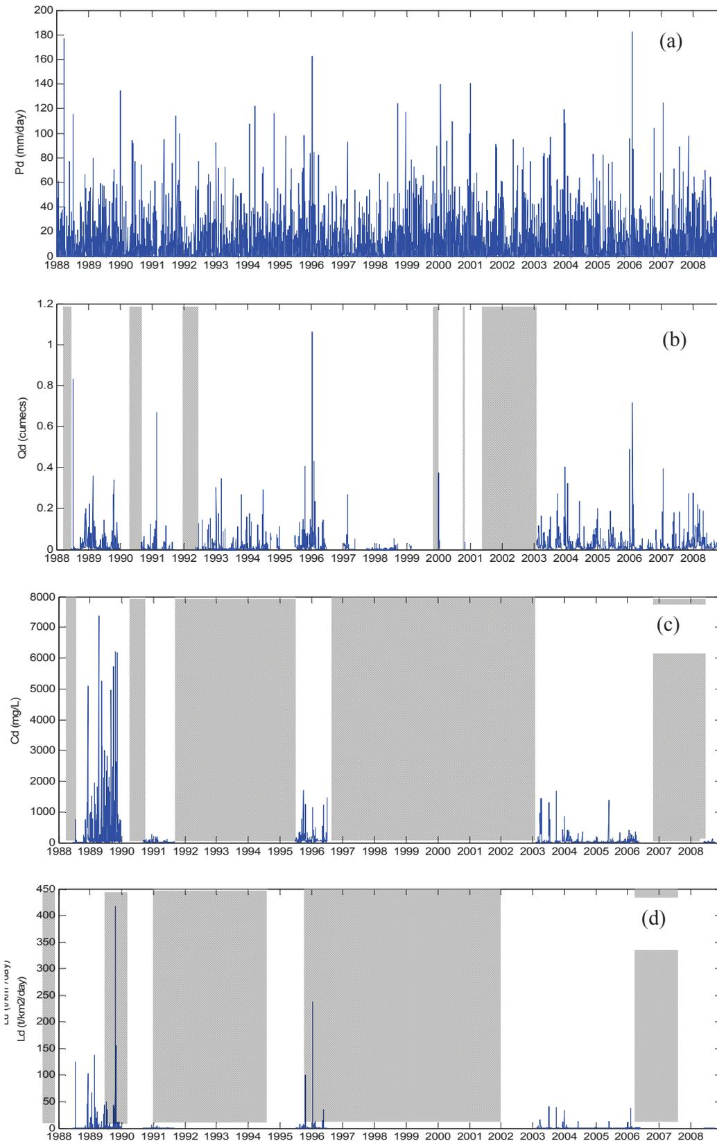
**Figure 15.3:** Quality assured time-series integrated at a daily resolution for (a) rainfall (mm day<sup>-1</sup>), (b) discharge (m<sup>3</sup> s<sup>-1</sup>), (c) suspended sediment concentration (mg L<sup>-1</sup>) and (d) suspended sediment load (t km<sup>-2</sup> day<sup>-1</sup>) over the period 1988-2008. Long periods without high quality data are shown with by stippling.
