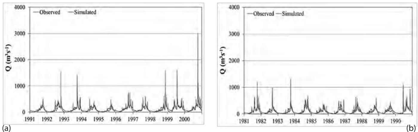
**Figure 10.3:** Observed and simulated hydrographs at the Cau 14 station for the (a) calibration and (b) validation periods
