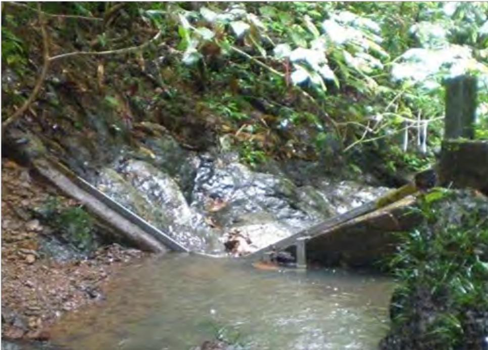
**Figure 15.2:** The 120° thin plate V-notch weir constructed at the Baru catchment outlet in January 1996. The original stilling well for the rated natural section monitored from 1988-1995 is shown on the right of the photograph.
